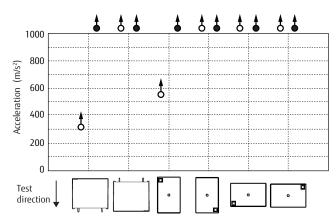
Test material: coil energized and de-energized Shock duration: 11ms (490m/s<sup>2</sup> or less)
