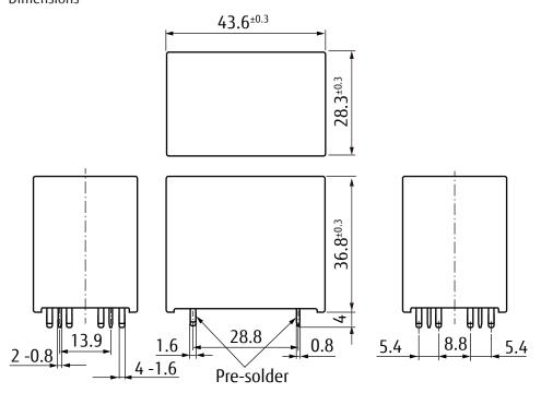
Note: Dimensions of the terminals do not include thickness of pre-solder.
