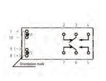
• PC board mounting hole layout (BOTTOM VIEW)
