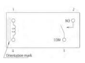
PC board mounting hole layout (BOTTOM VIEW)
