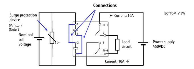
**Note 1**: In case 2 coils are connected in series, connect coil terminal #2 to #3 on PCB circuit. In case 2 coils are connected in parallel, connect coil terminal #1 to #3 and connect coil terminal #2 to #4 on PCB. Regarding terminal number, refer to schematics data.
