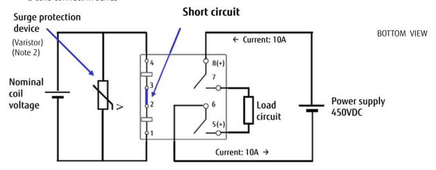
Load circuit contact terminals have polarities (+) and (-). Coils do not have polarity.
