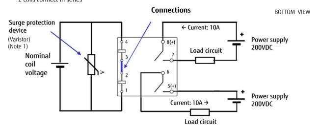
Load circuit contact terminals have polarities (+) and (-). Coils have no polarity.
