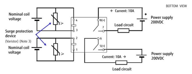
**Note 1**: In case 2 coils are connected in series, connect coil terminal #2 to #3 on PCB circuit. In case 2 coils are connected in parallel, connect coil terminal #1 to #3 and connect coil terminal #2 to #4 on PCB. Regarding terminal number, refer to schematics data.
